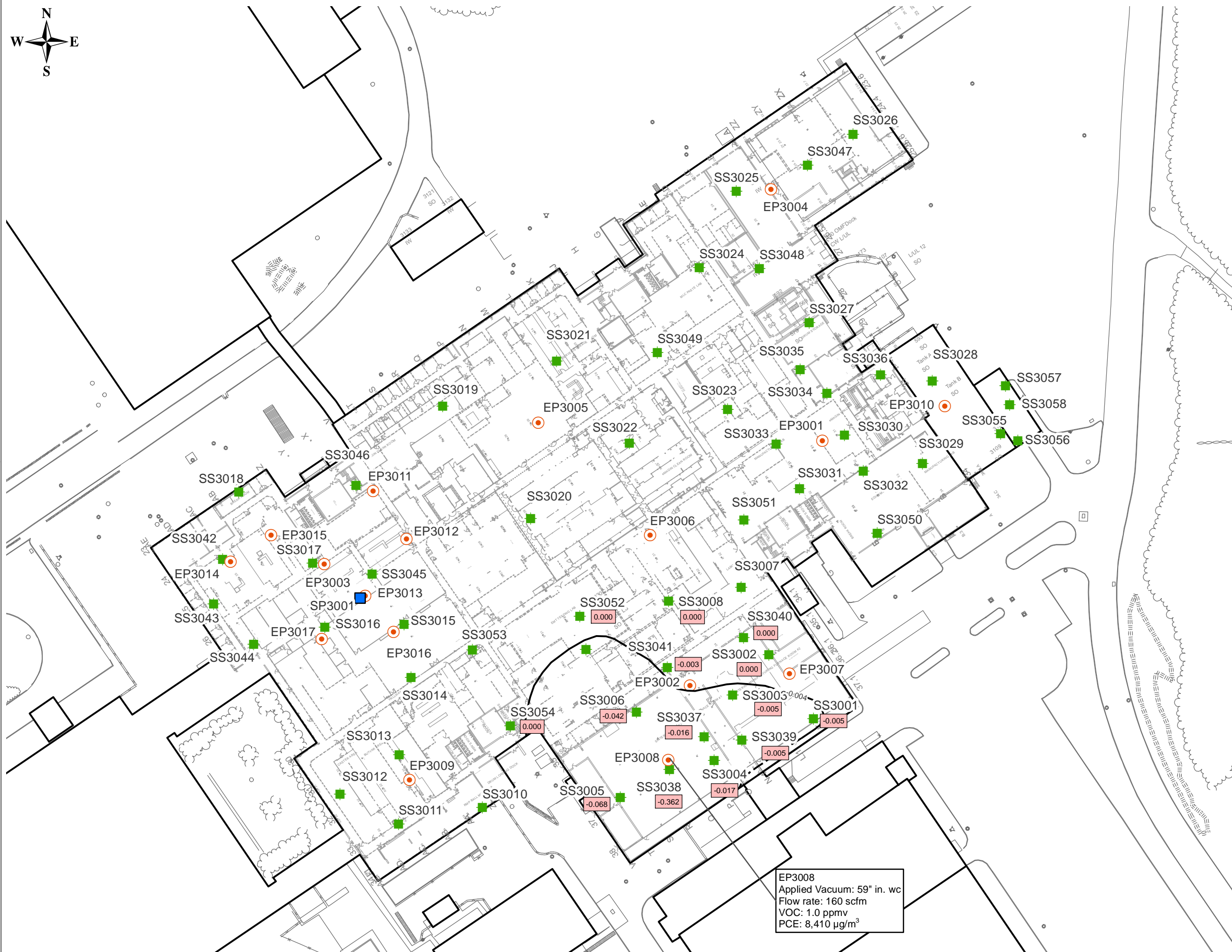
Subslab Pressure Response to Vapor Extraction Testing
