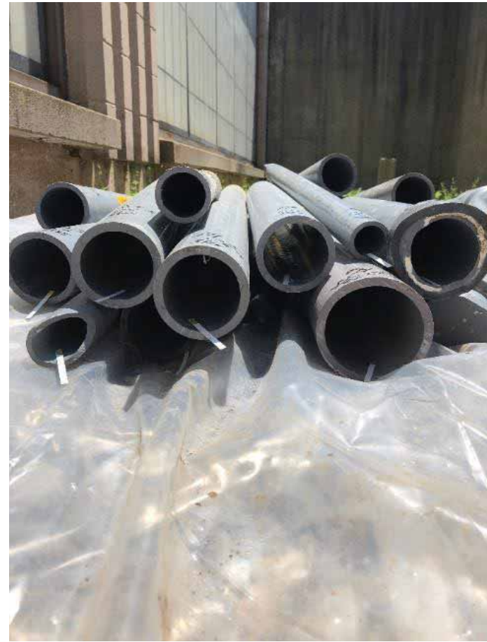
Industrial Waste Pipe Sampled And Inspected After Being Cleaned
