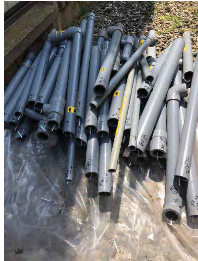
Industrial Waste Pipe Sampled And Inspected After Being Cleaned
