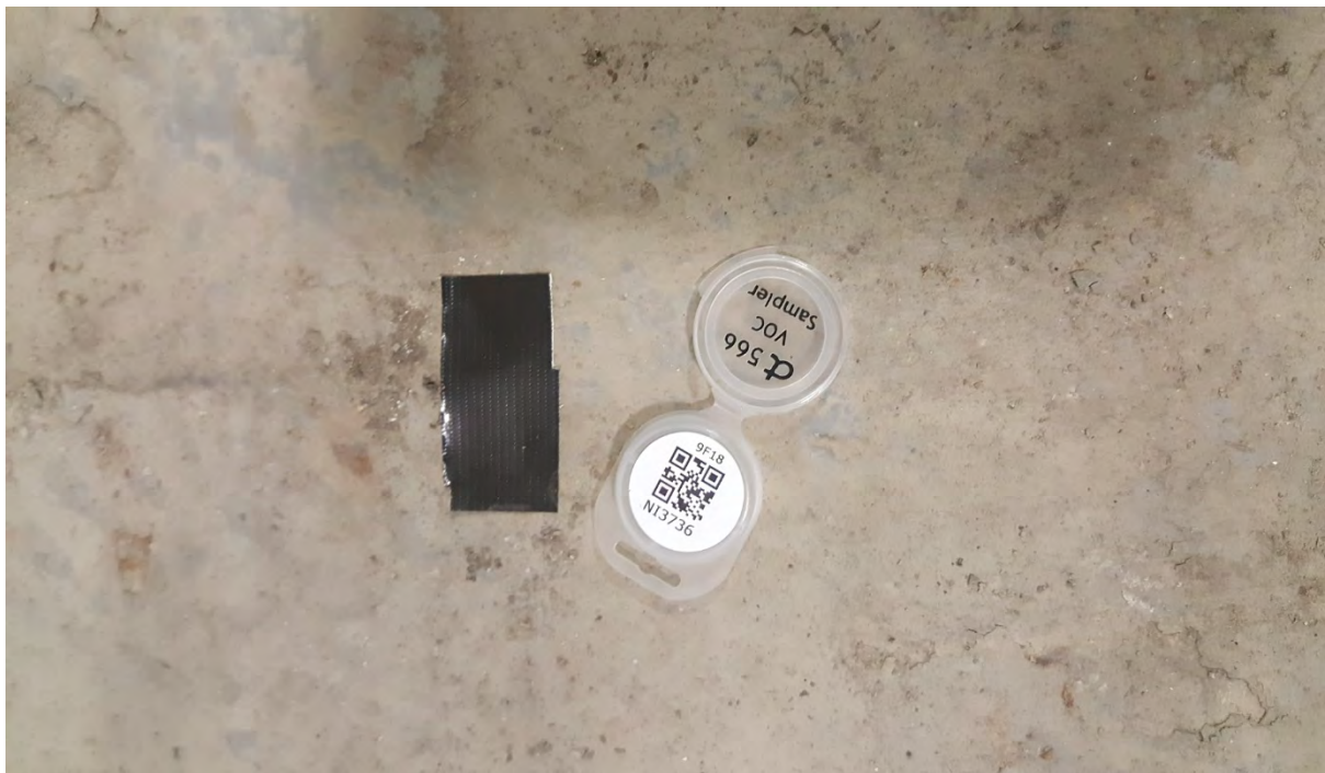
Photo 7: Close-up of passive sampler deployed face-down on floor slab
