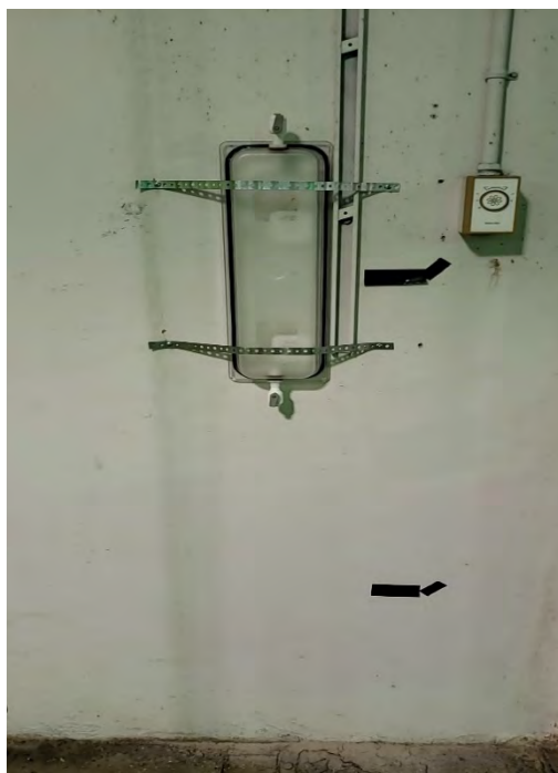
Photo 14: Flux chamber fastened to wall with straps
