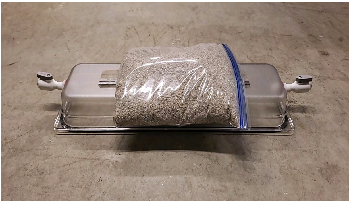
Photo 13: Close-up of flux chamber set up on floor being held down with a weight
