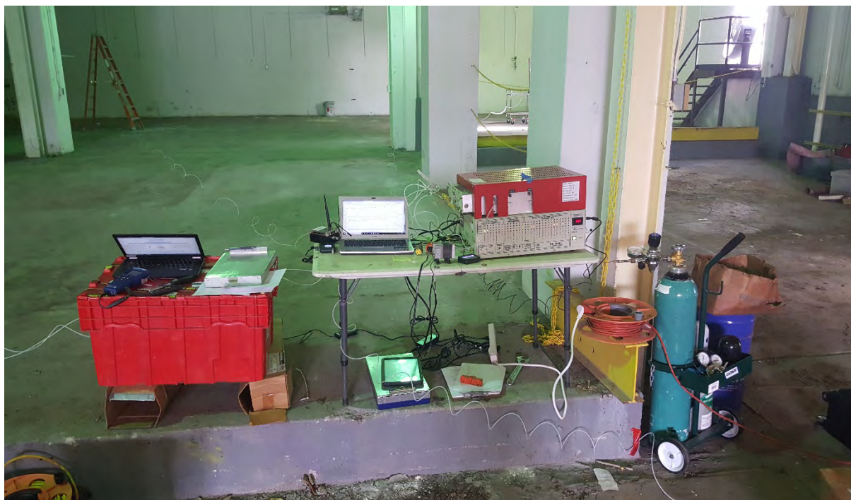
Photo 8: GC-ECD set-up during pressure testing
