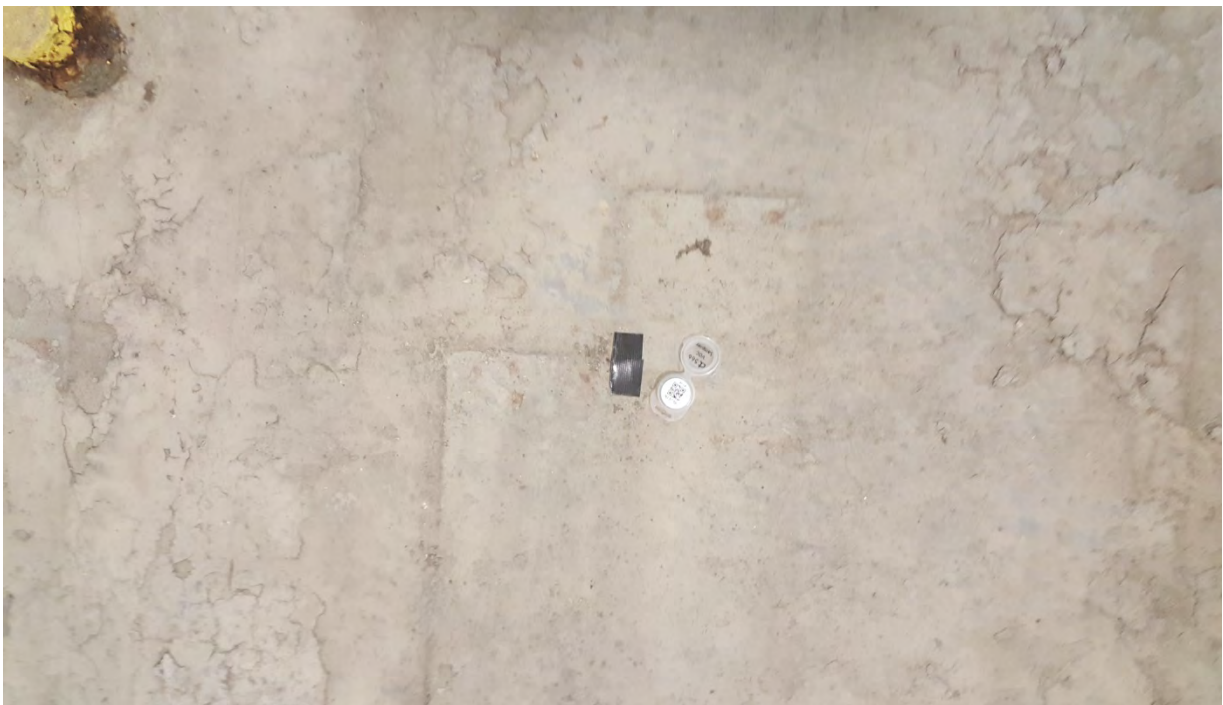
Photo 6: Passive sampler deployed face-down on floor slab
