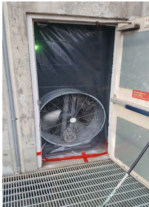
Photo 10: Fan and surrounding plastic during positive pressure test
