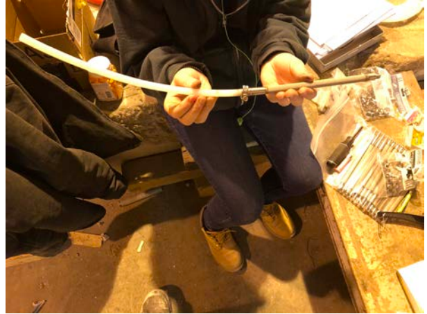
Microwell screen and tubing for monitoring point.
