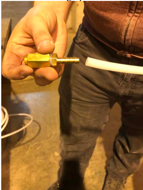
Monitoring point brass fitting assembly.
