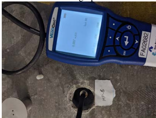
MP-6 Vacuum reading (-0.007 in WC)
