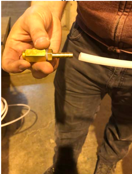
Monitoring point brass fitting assembly.
