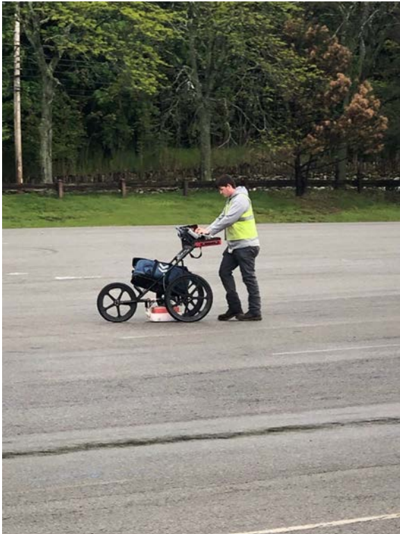
Photograph #1 GPR mark out
