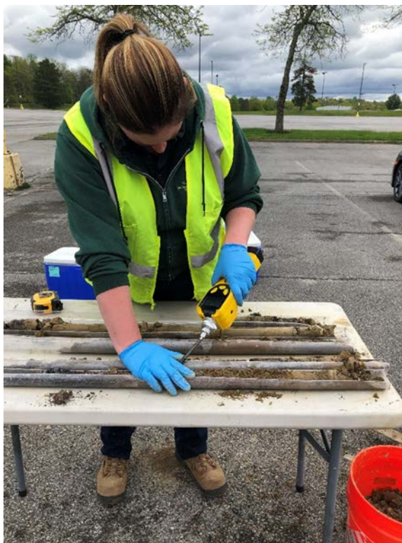
Photograph #6 PID reading soil sample
