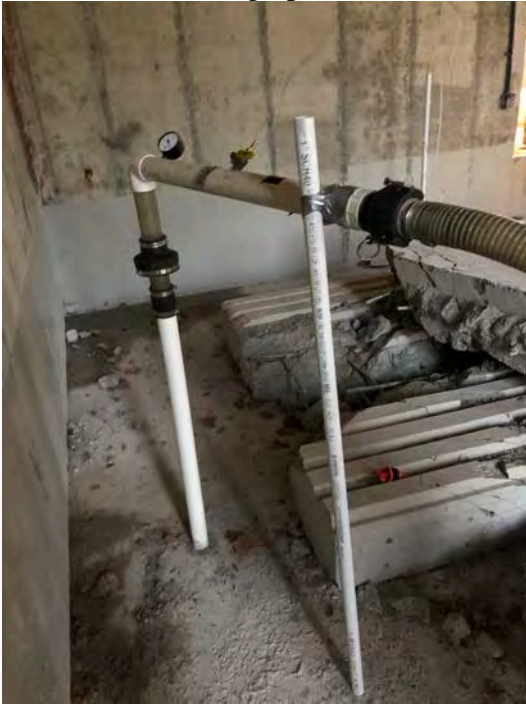
Vapor extraction well point connected to blower during pilot test
