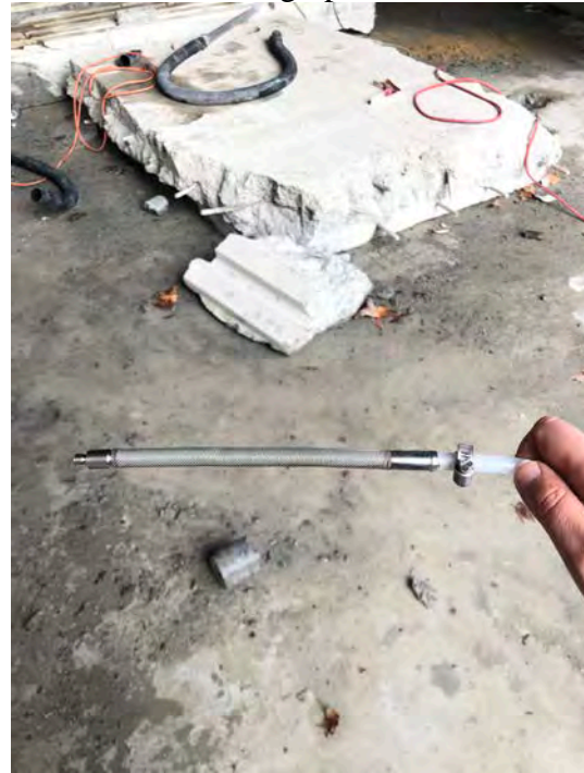
Microwell screen for monitoring point
