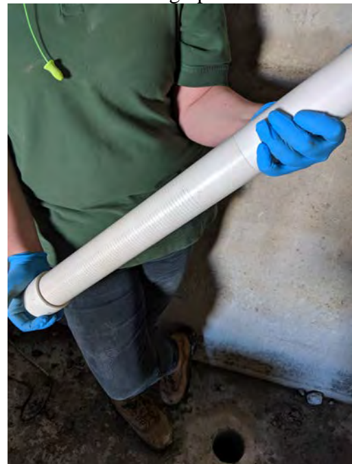
Vapor extraction well point slotted PVC pipe
