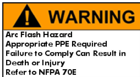
Minimum arc flash label example
