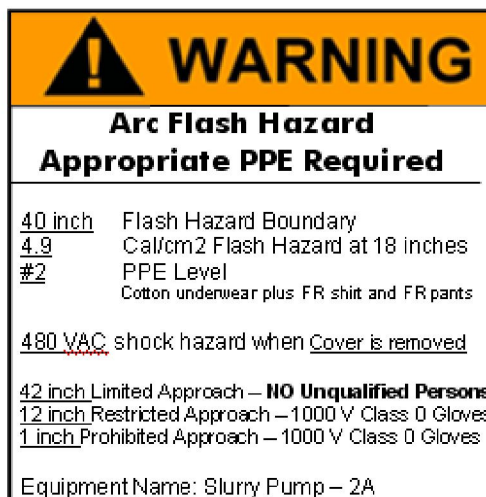
Detailed (preferred) arc flash label example
