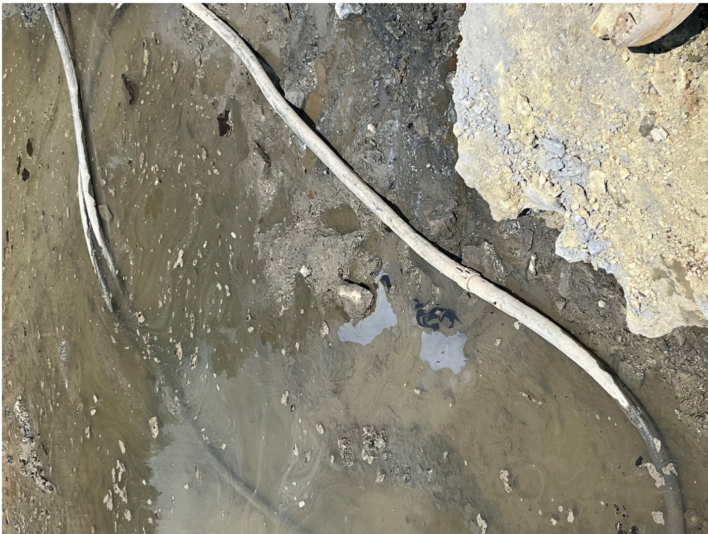
Blebs and stringers in groundwater within former holder excavation.
