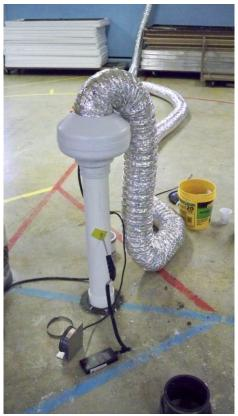
Extraction Point Setup for Communication Test – Including Anemometer and Magnehelic Monometer
