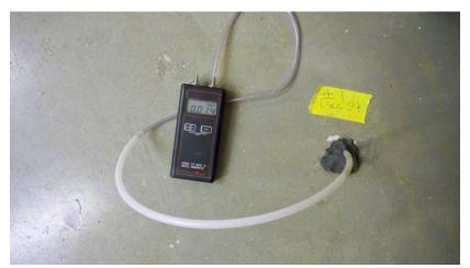
Vacuum Point Measurement for Communication Test Using Digital Micro-Monometer
