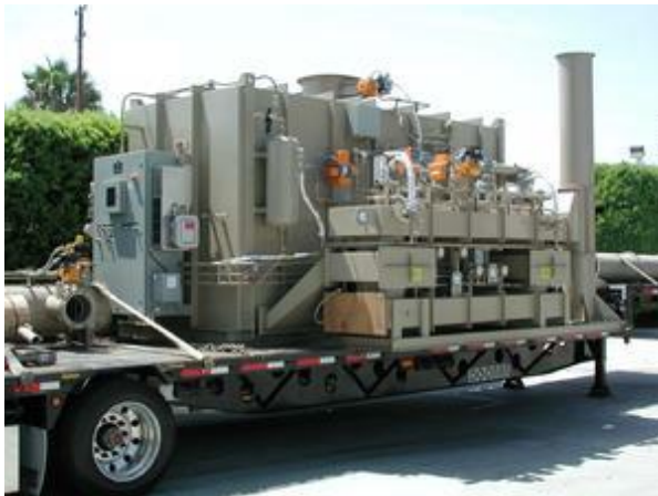
RETOX 4,000 RTO for AMINE GAS STRIPPING
