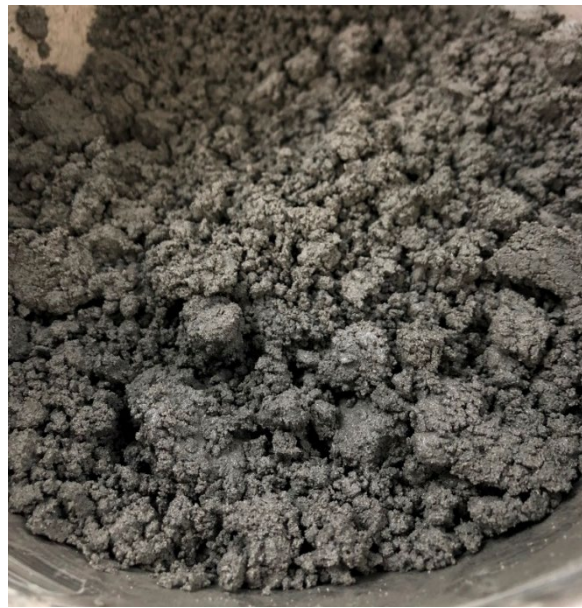
Picture 2: After site soil / sand blending
