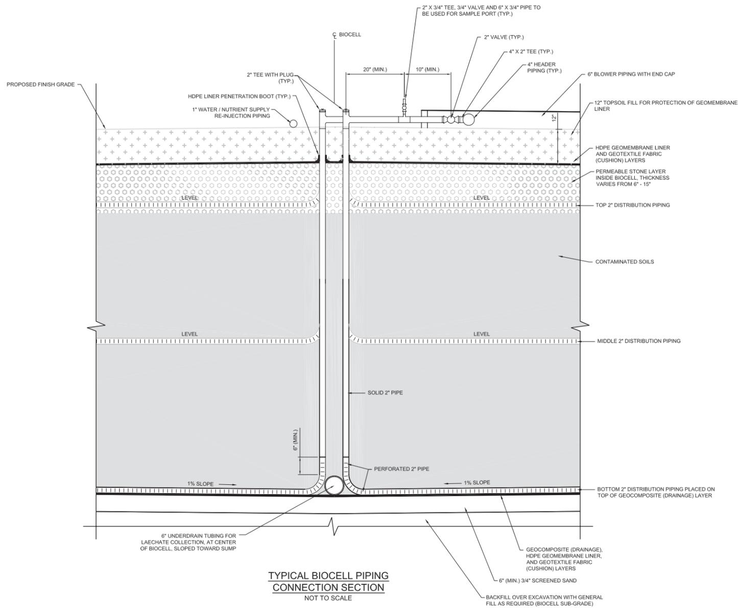
**TYPICAL BIOCELL PIPING CONNECTION SECTION**
