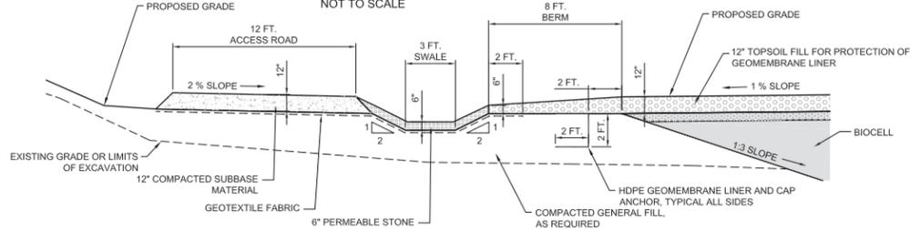
**TYPICAL ACCESS ROAD AND LINER ANCHOR TRENCH DETAIL**
