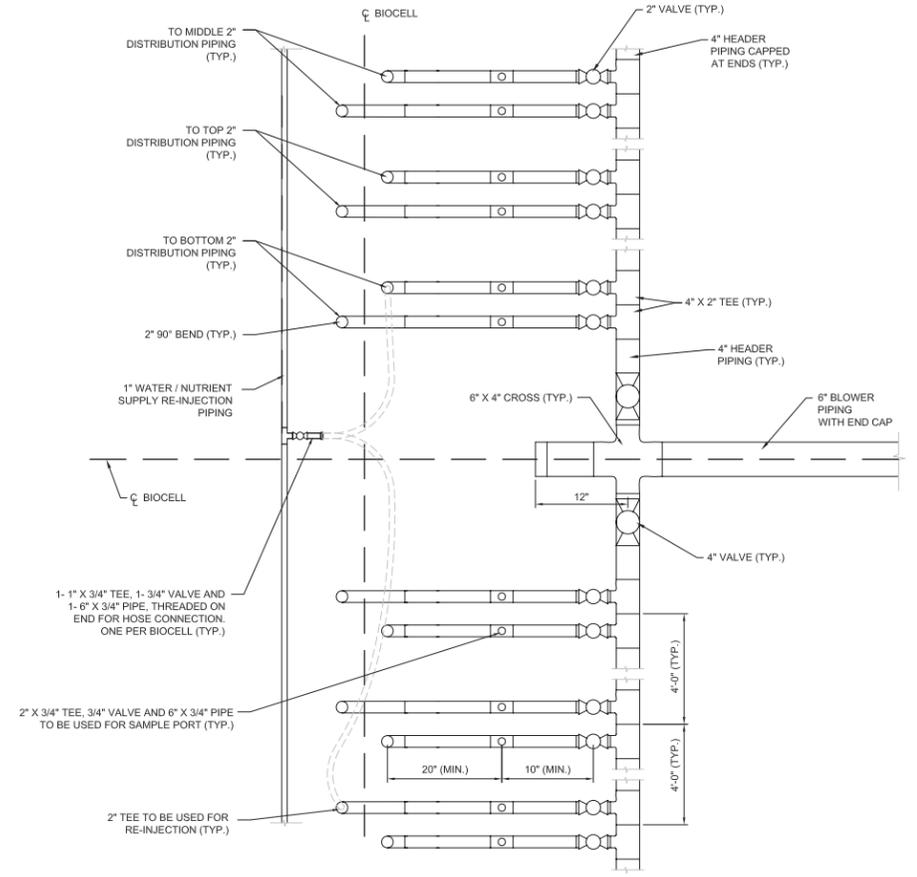
**TYPICAL BIOCELL MANIFOLD PIPING DETAIL**
