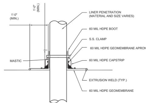
**HDPE LINER PENETRATION DETAIL**
