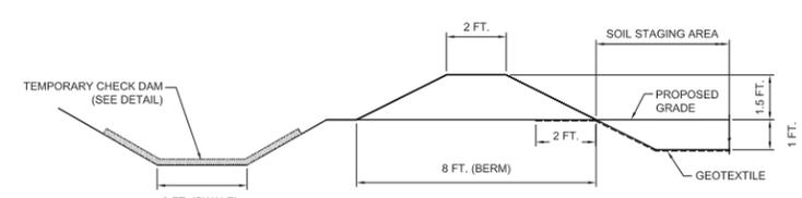
**DRAINAGE SWALE AND DIVERSION BERM DETAIL**
