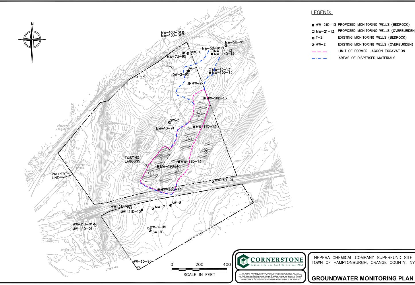
■ MW-21D-13 PROPOSED MONITORING WELLS (BEDROCK) □ MW-21-13 PROPOSED MONITORING WELLS (OVERBURDEN) EXISTING MONITORING WELLS (BEDROCK) EXISTING MONITORING WELLS (OVERBURDEN) LIMIT OF FORMER LAGOON EXCAVATION AREAS OF DISPERSED MATERIALS
