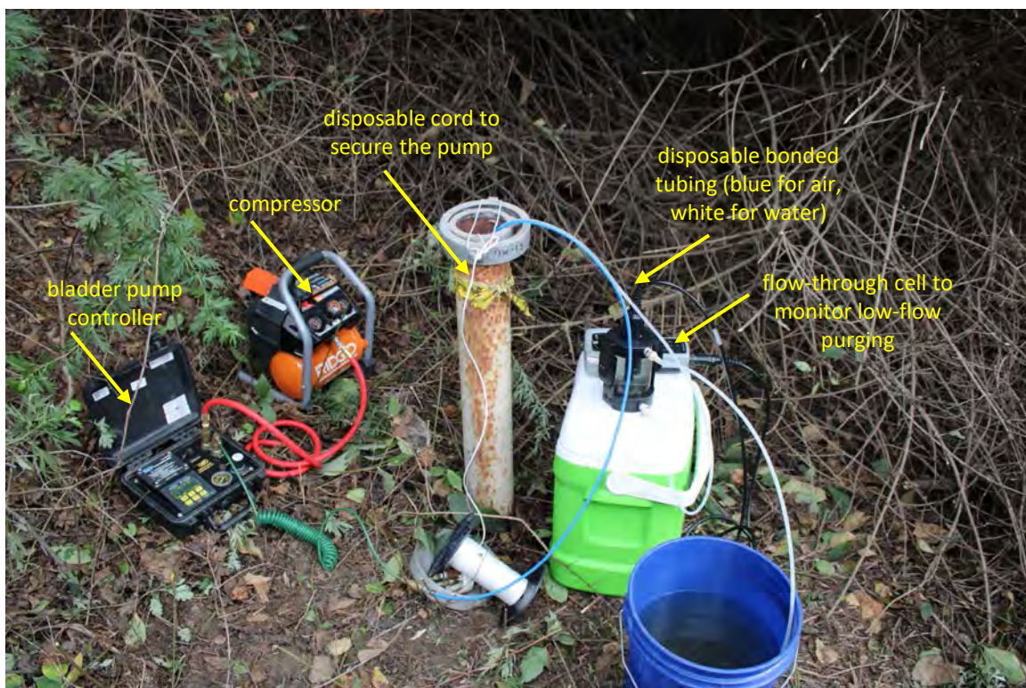
A downhole stainless steel bladder pump with a single use PE bladder was used to sample OW-19. Compressed air was used to pump the water.
