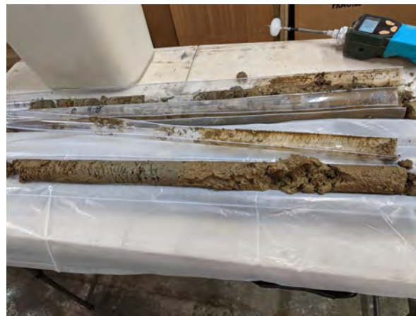
4. Typical cut boring sleeve
