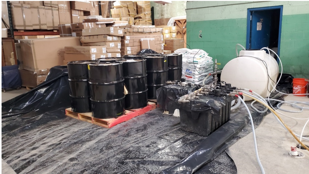
Photograph 3. ISCO injection equipment staged within containment.
