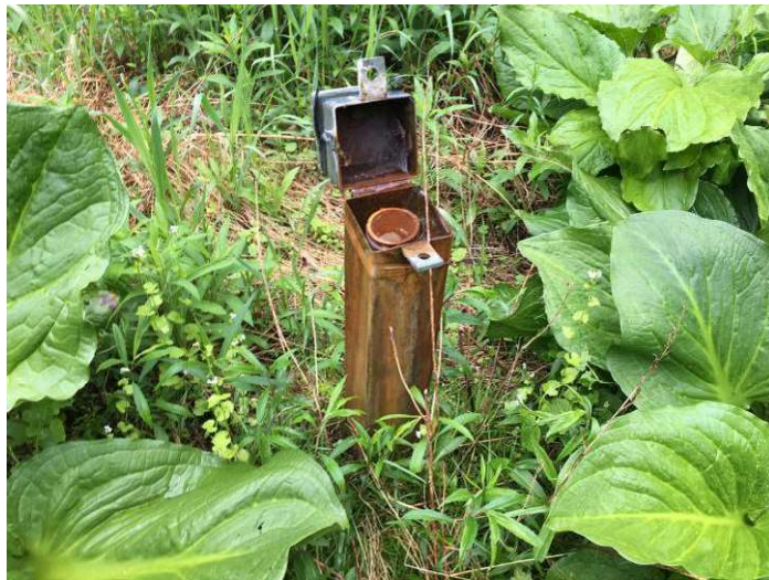
Photo 6: View of well MW-7. Artesian conditions noted in well and staining on casing due to artesian flow out of monitoring well.
