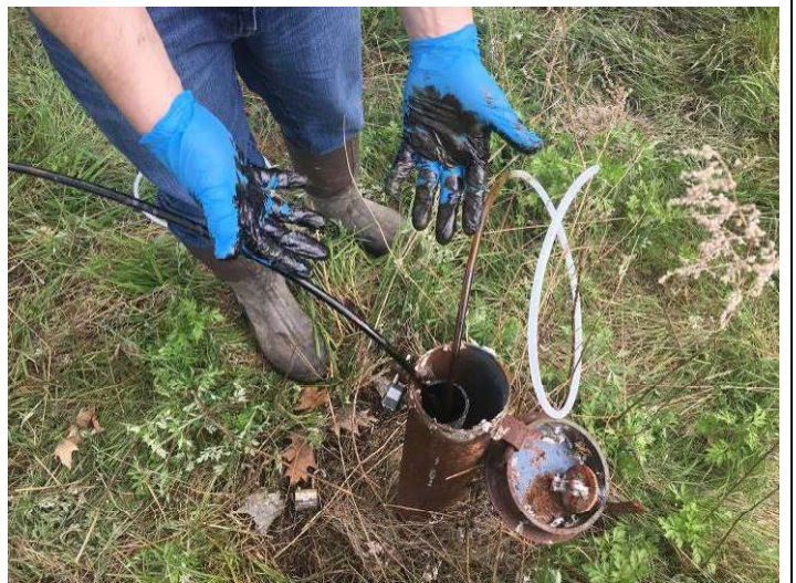
Photo 4: Looking south. View of product found on tubing placed into MW-4R.
