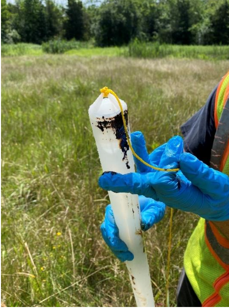
Photo 7: View of bailer after being remove from MW-4R.
