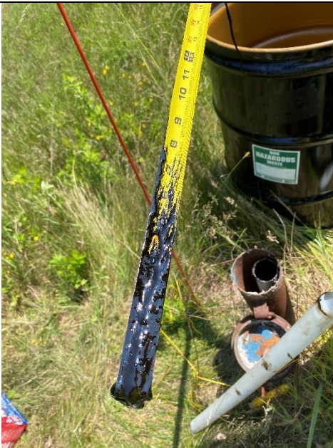
Photo 9: View of viscous product from the bottom of MW-4R on measuring tape.
