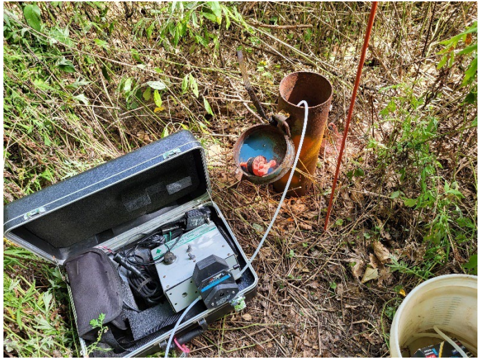
Photo 8: View of sampling activities at MW-4DR using low-flow methodology. Facing south.
