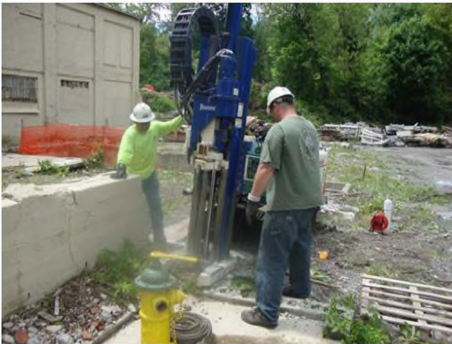
Photo 2 – Collecting pre-treatment baseline soil samples
