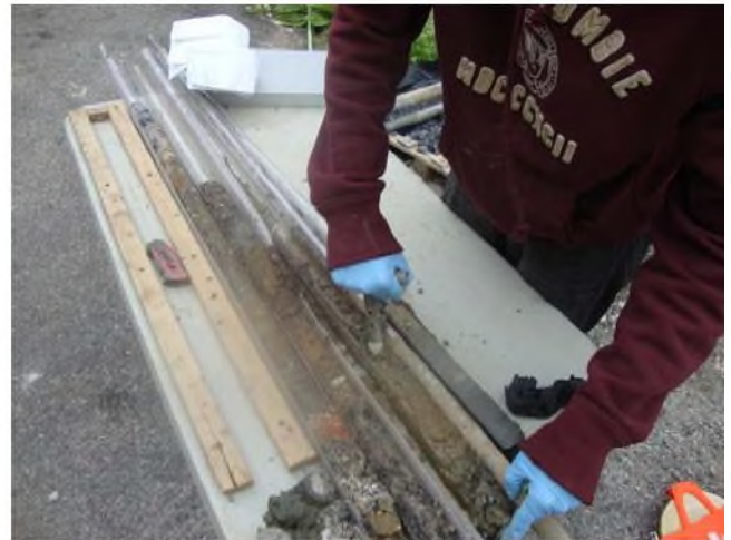
Photo 3 – Baseline soil samples and cores
