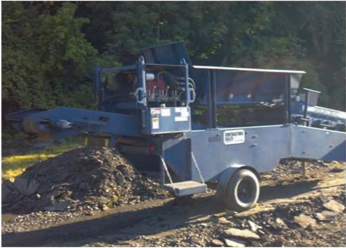
Photo 8 – Soil going through screener to remove large debris
