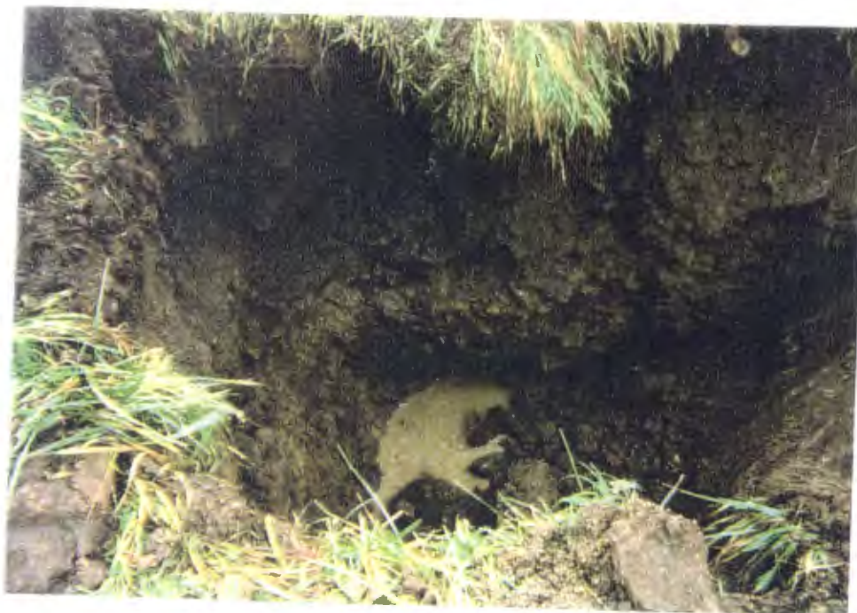
Photograph 2 Test Pit 01 - Groundwater at 4 ft., No landfill debris
