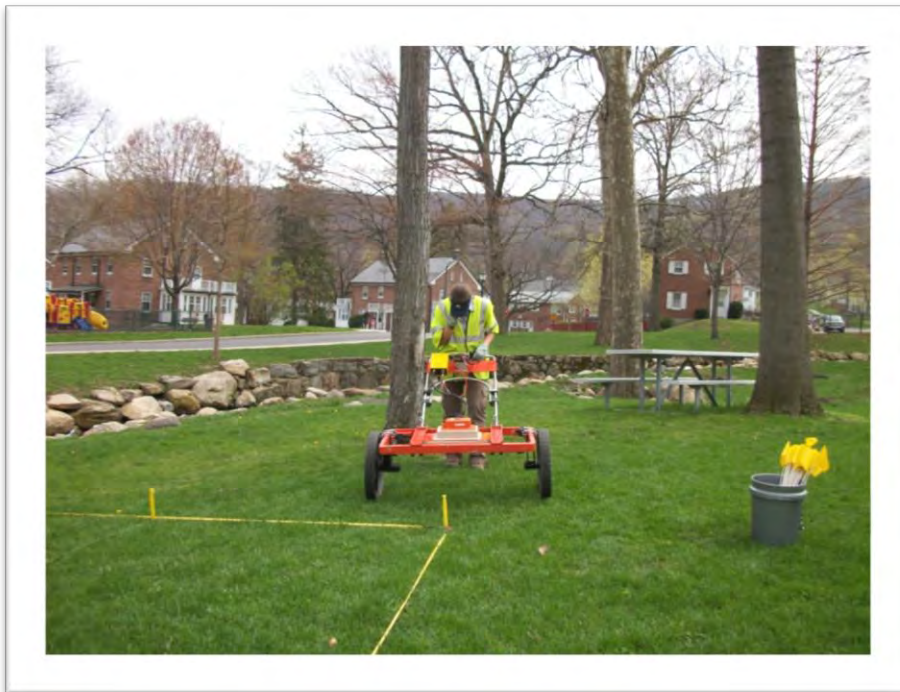
Geophysical Technician collecting DGM data at grid LR-09 in Lusk Reservoir MRS.
