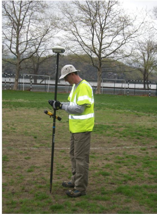
Geophysical Technician testing RTK GPS at Target Hill MRS.
