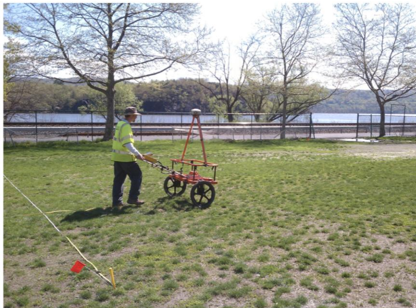
Geophysical Technician collecting DGM data at Target Hill MRS.
