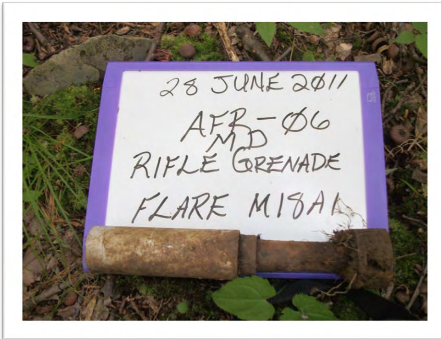
Rifle Grenade Flare M18A1 (munitions debris) recovered from grid AFR-06 in Artillery Firing Range MRS.
