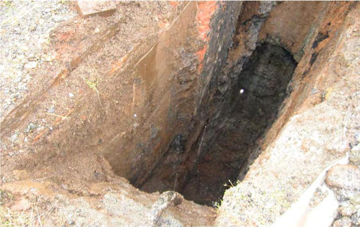
Photo 5: PDI-TP-3 black staining between 6' and 16' bgs. Brick covered by cement holder wall on the left.
