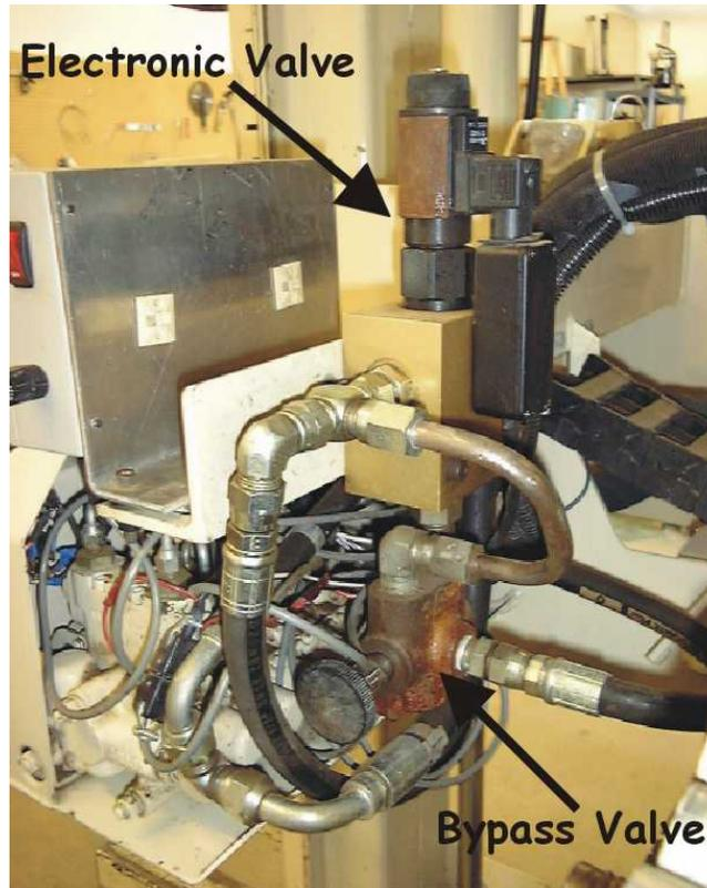
The operator can now hold down the leftmost probe control lever. The default probe rate is 2cm/sec. **The operator should be prepared at any time to begin hammering to prevent the probe from lifting too far off of the ground.** Continue probing to desired depth by cycling the probe up, adding a rod and pushing it at a controlled rate.
