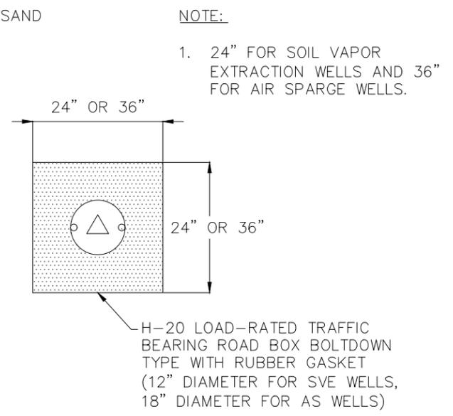
**SOIL VAPOR EXTRACTION/AIR SPARGE WELLHEAD MONUMENT DETAIL**
