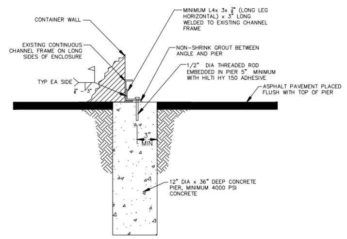
**EQUIPMENT ENCLOSURE ANCHORING DETAIL**
