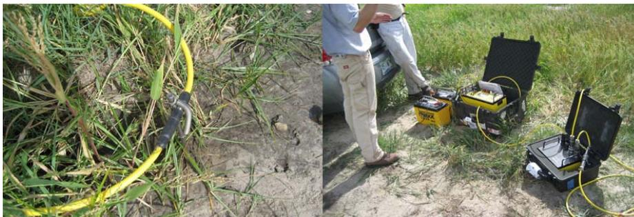
Once the electrodes and cables are deployed, the survey will begin. The unit is powered by two deep cycle marine batteries. Two types of surveys are planned for each survey line. The first is RES and IP using a dipole-dipole array. The second is the Inverse Schlumberger array which, when combined with the dipole-dipole array, improves the resolution of laterally continuous lithologic features.
