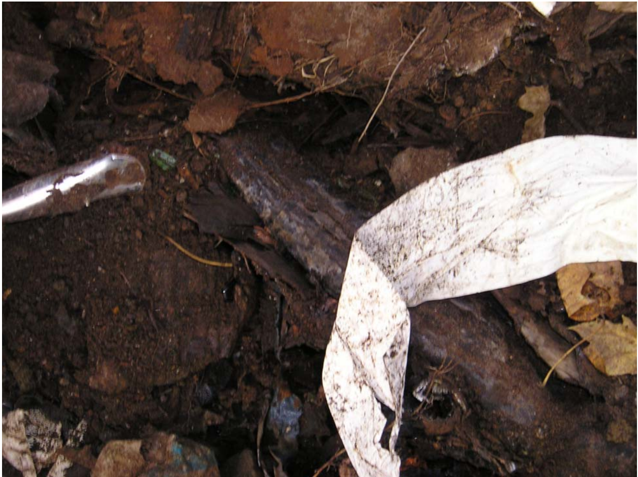
Photo 4: Close up of drum where sample TP-15B was collected. Drum was approximately 3 feet below grade. Soil sample TP-15B Soil was collected near the silver object. PID reading of waste approximately 600 ppm and the soil approximately 100 ppm.
