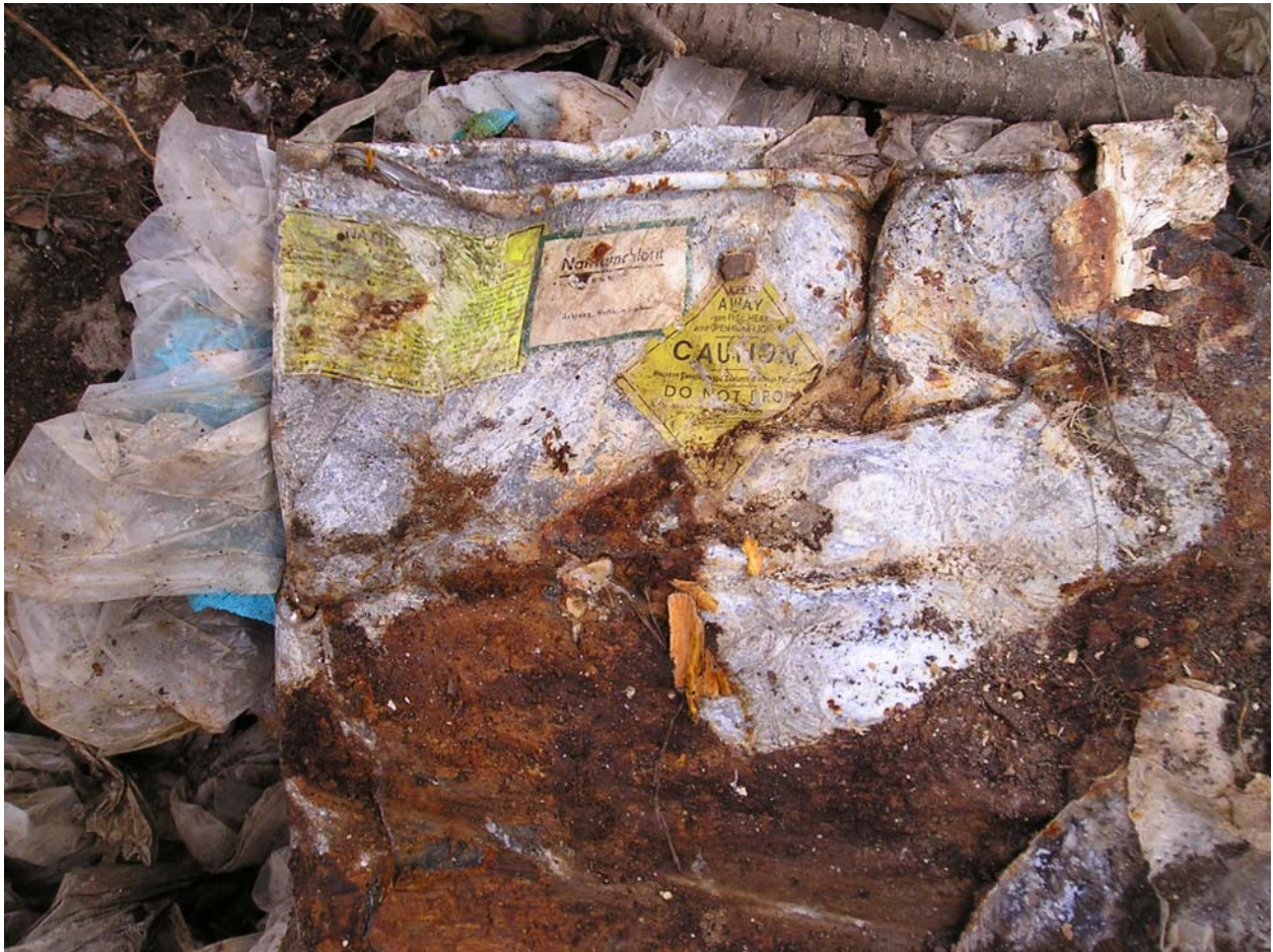
Photo 2: Metal drum found in test pit TP-15. Found approximately 4 feet below grade in test pit.
