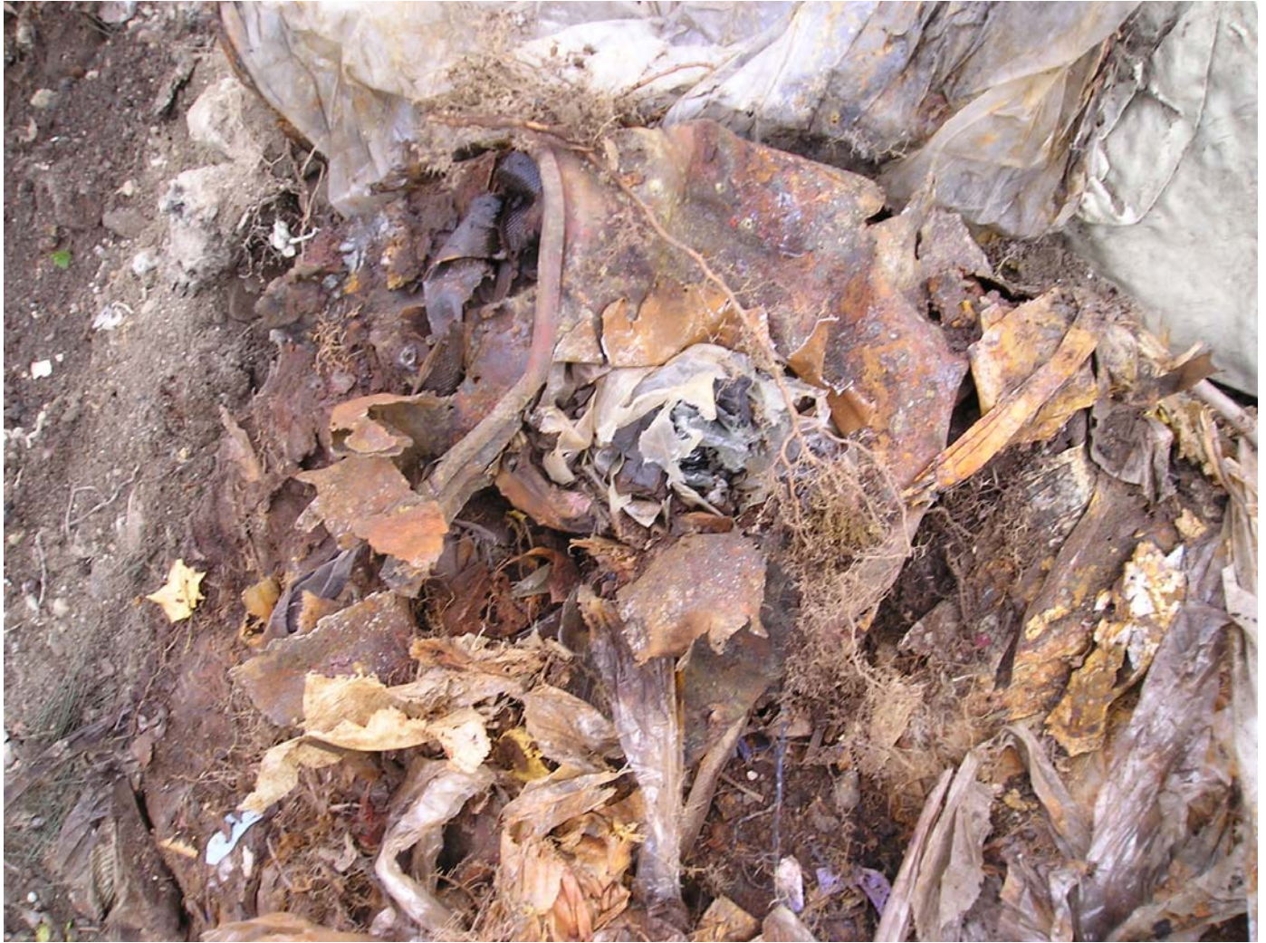
Photo 1: Close up of drum where sample TP-15A was collected. Drum was found approximately 3 feet below grade in test pit. PID reading >9999 ppm.
