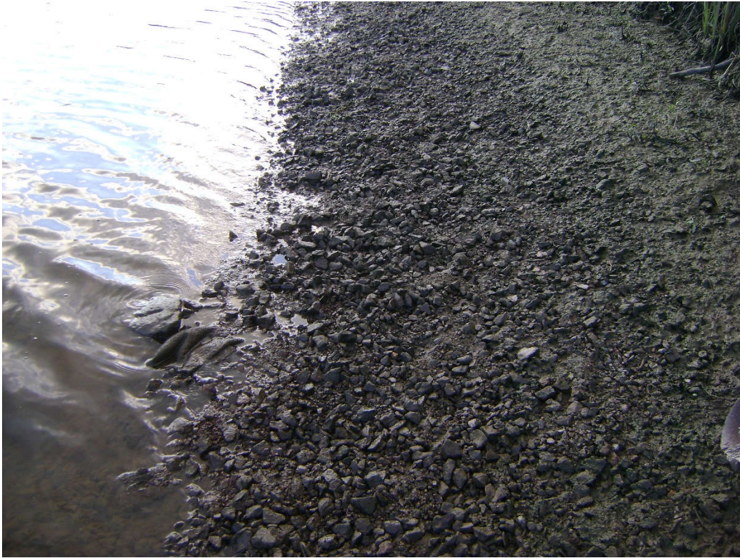
Photo 1 – Bub 1 – (photo taken September 20, 2021) No change since last visit. Several small springs parallel to shore, still underwater at low tide. Springs coming from edge of GCL close to surface. No soft feel to ground anywhere in this area.
