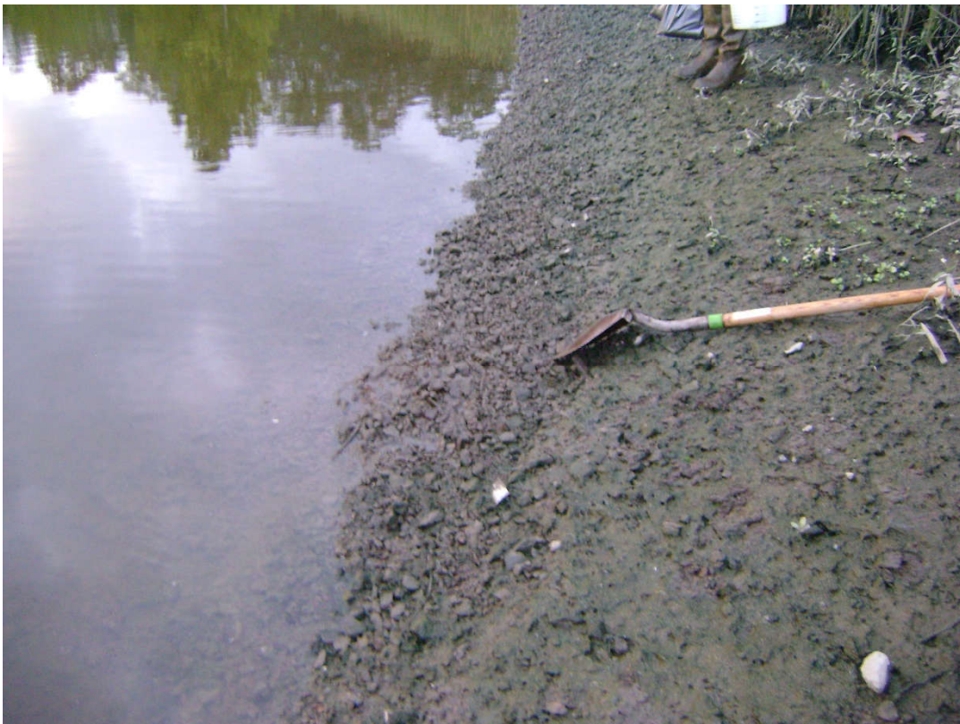
Photo 2 – Bub 2 – (photo taken September 20, 2021) No change since last visit. Small amount of water draining from stone, indicated by shovel head. No soft feel to ground anywhere in this area.
