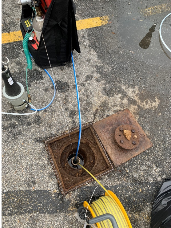
TRC purging MW-02D with a bladder pump.
