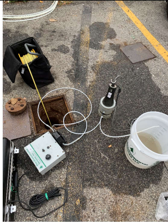
TRC purging MW-02D with a peristaltic pump.
