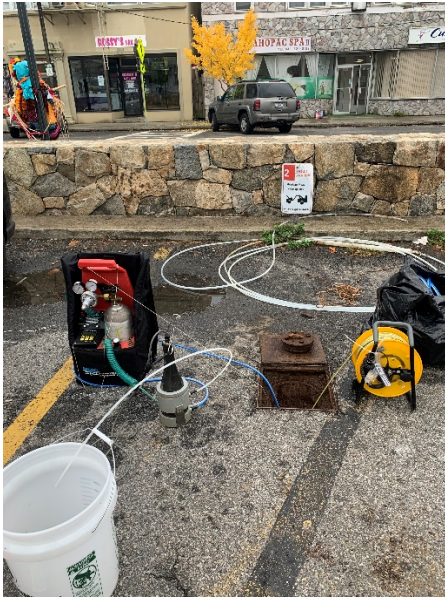
TRC sampling set up at MW-02D.
