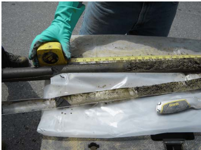
Soil sample from boring #2 showing the top of the clay layer. (Interval from 12 to 14 feet).
