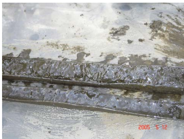
Coal tar at boring #8 (interval from 10 to 12 feet).
