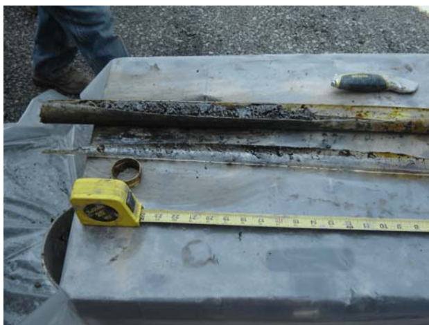
Coal tar in boring #5 (interval from 4 to 6 feet).
