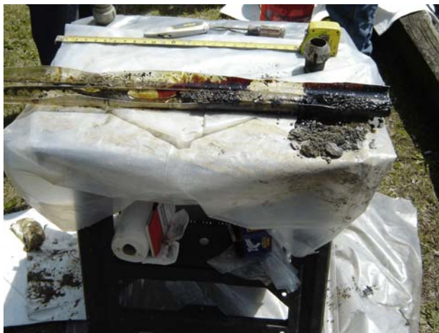
Coal Tar in boring #3 (interval from 4 to 6 feet).
