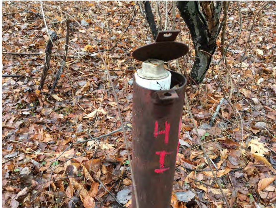
Photograph 21: Monitoring well 4-I (utilized for depth to water measurements only) is not able to close and lock (north to south).
