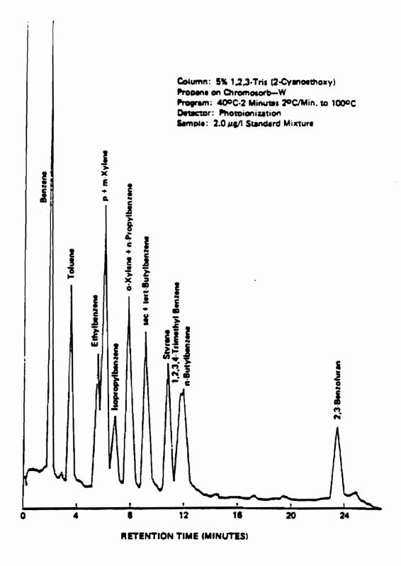
Figure 2. Chromatogram of aromatic volatile organics (column 2 conditions).
