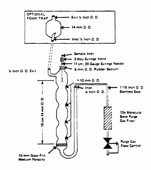
Figure 1. Purging chamber.
