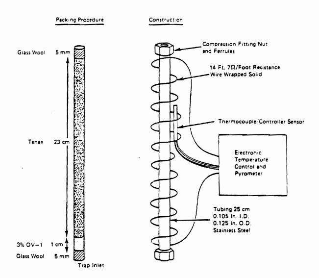
Figure 3. Trap packing and construction for Methods 8020 and 8030.
