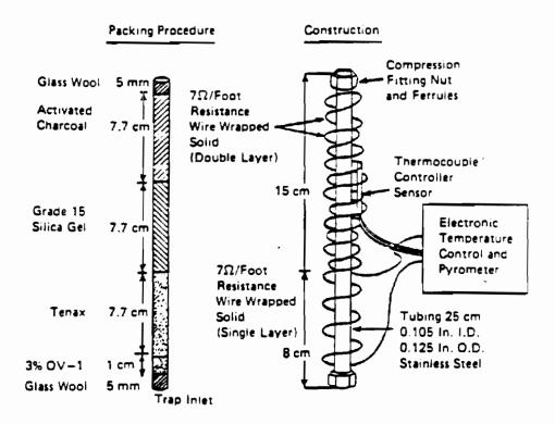
Figure 2. Trap packings and construction for Method 8010.
