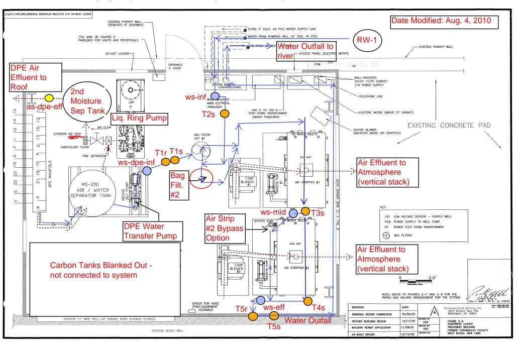
P&T System Flow Diagram
