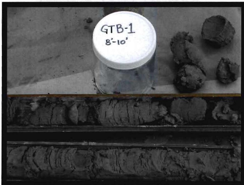
Soil Boring GTB-1, 8-10 Feet Below Ground Surface. Grey Clay With Frequent mm Scale Silt Beds. No Visual Impacts Noted at Water Table.
