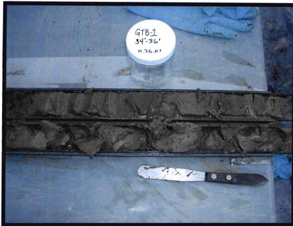
Soil Boring GTB-1, 34-36 Feet Below Ground Surface. Brown to Light-Brown Silt and Clay. No Visual Impacts Noted at End of Boring.
