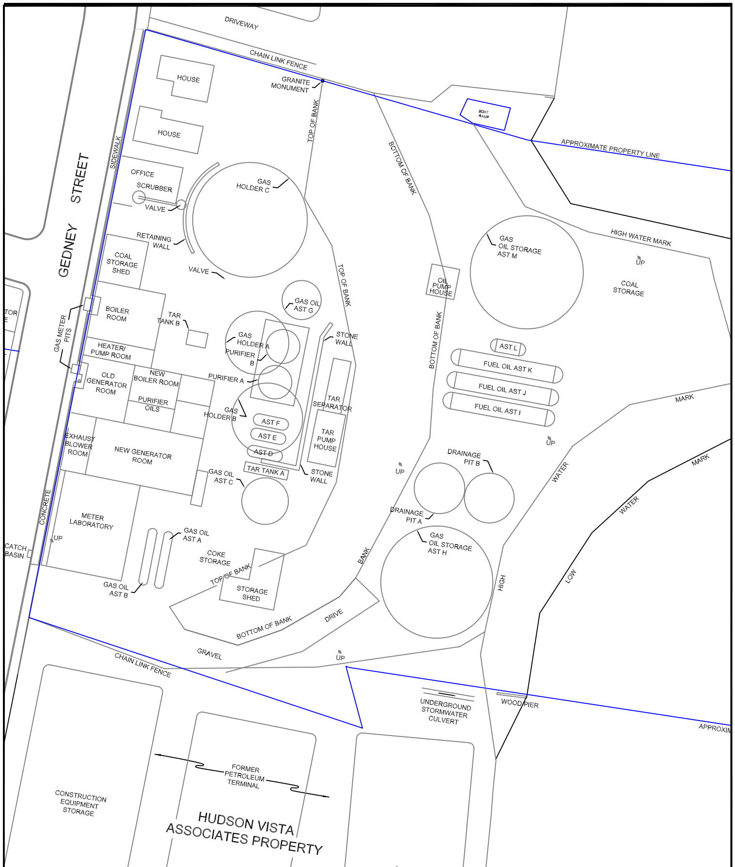
NYACK GAS PLANT SITE (OU-1) NYACK (C), ROCKLAND COUNTY, NEW YORK SITE NO. 3-44-046 HISTORIC STRUCTURES
