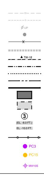
LEGEND: 5-FOOT INTERVAL CONTOUR 1-FOOT INTERVAL CONTOUR UTILITY POLE WOODEN PILE CHAIN LINK FENCE UNDERGROUND STORMWATER CULVERT WETLAND DELINEATION MEAN HIGH WATER LINE (MHW) MEAN LOW WATER LINE (MLW) PROPERTY LINE OU2 BOUNDARY ISS AREA DREDGE AREA ZONE DREDGING TARGET DEPTH ISS TARGET DEPTH JET GROUTING PRE-CHARACTERIZATION SONIC DRILL PRE-CHARACTERIZATION VIBRACORE SAMPLE MONITORING WELL (TO BE ABANDONED)
