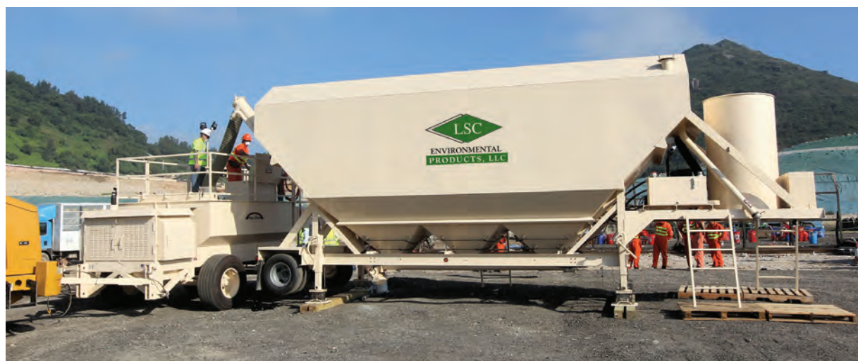
Horizontal silo loading powdered product into a Posi-Shell Applicator.
