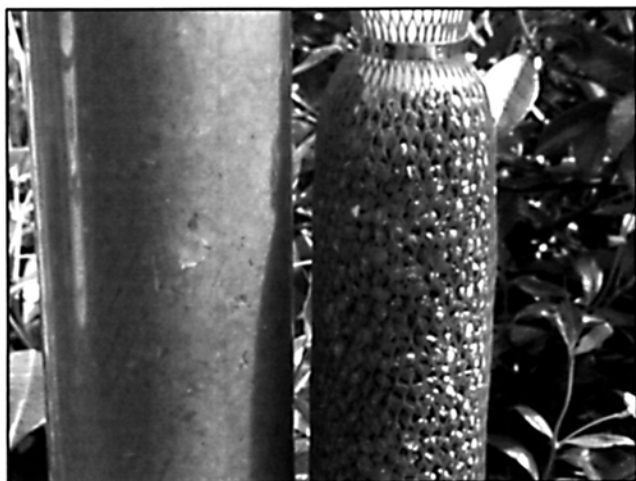
Figure 7. Bentonite packer (right) prior to insertion in a borehole. To left, bentonite packer after it has hydrated and swelled.
