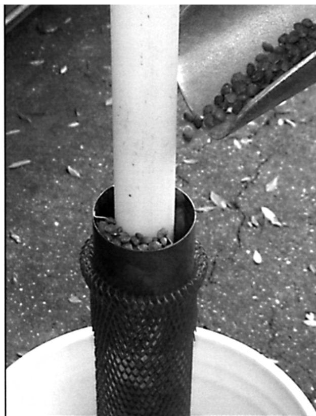
Figure 6. Stainless-steel form used to construct bentonite packers.
