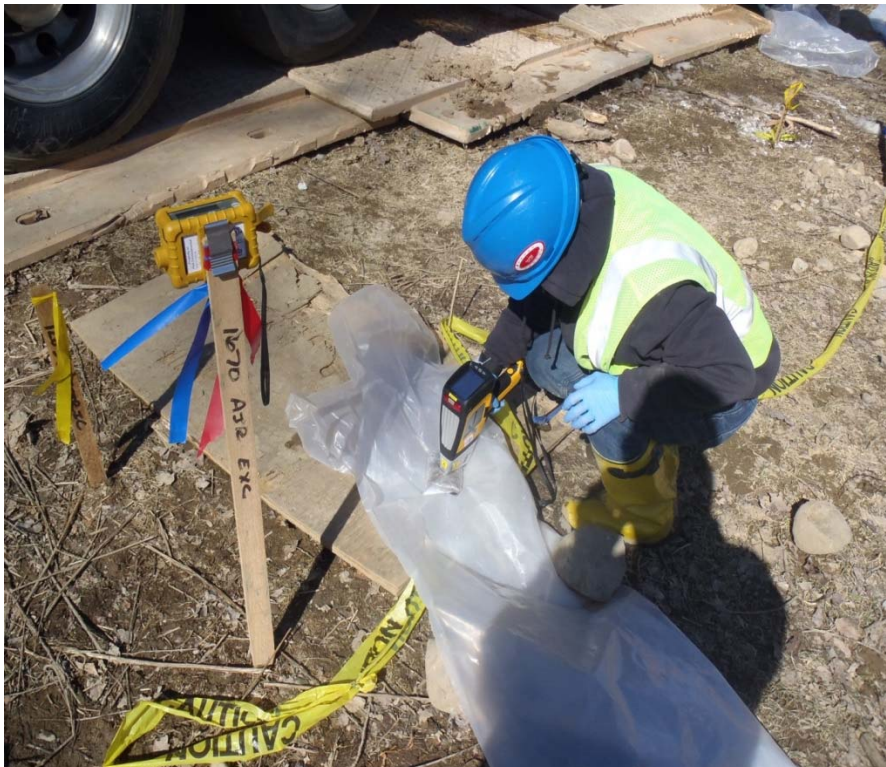
Figure 4: Using XRF to analyze soil samples for metals
