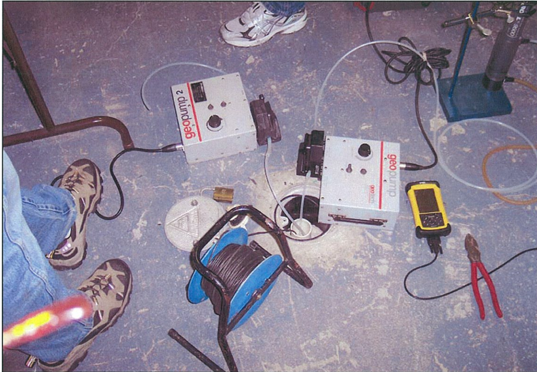
Picture below: Low-stress sampling set up completed on 10/30/06.
