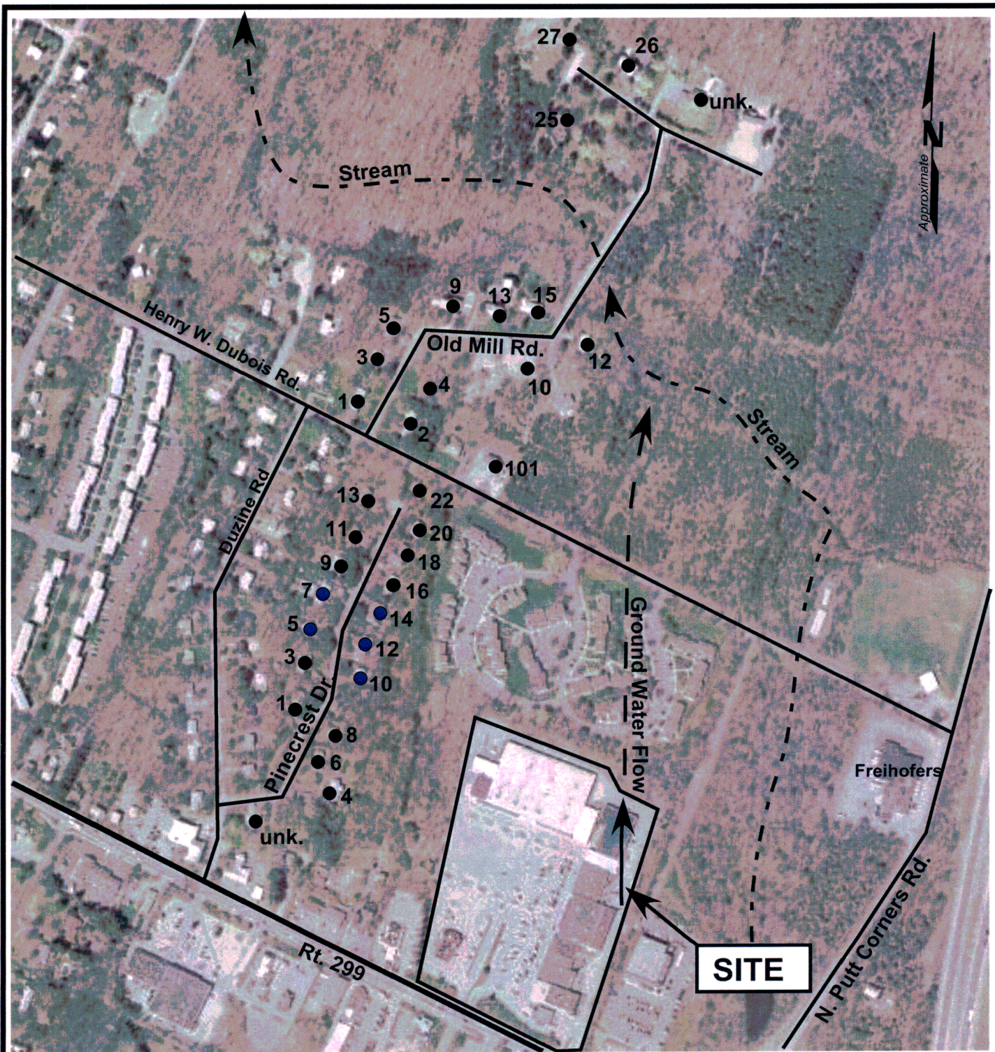
FIGURE 5 Well Survey and Ground Water Flow Map
