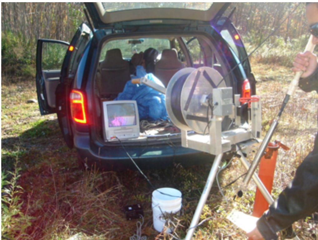
Video logging pre-existing wells, November 2007 (Photo from TtEC files, 2007)
