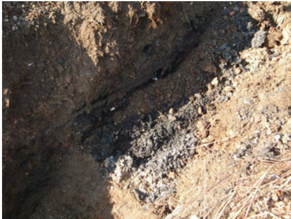
Test Pit TP-02, excavated November 5, 2007, black staining, sulfide odor noted (Photo from TtEC files, 2007)
