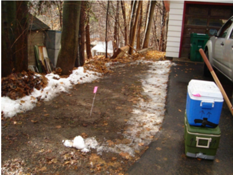
Residential Soil Sample RSS-02 Location, sampled on December 5, 2007, Lead and PCB concentrations exceed Residential SCOs) (Photo from TtEC files, October 2007)
