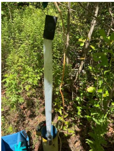
Photo #5: View of EPA-09 along with newly installed hydrosleeve. Facing west
