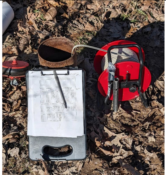
SVE Wells Purged, Sampled and Monitored for Recharge.
