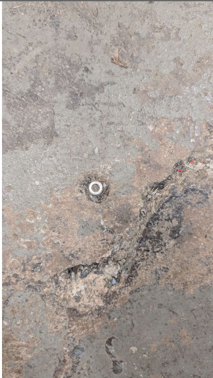
Photo 10: SGP-11 is damaged. Vacuum = 0.028 inWC
