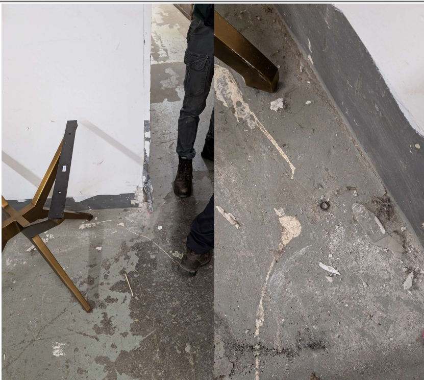
Photo 8: Port-1 in main hallway. Underneath leather couch. Vacuum = 0.000 inWC
