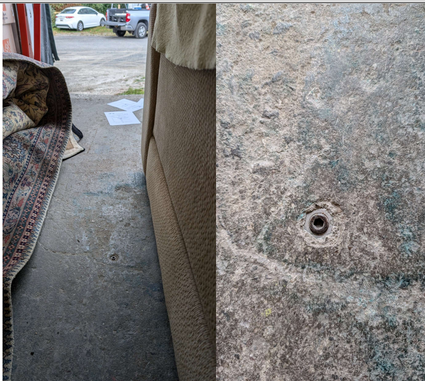
Photo 6: SGP-8. Northern overhead door on west side of the building. Vacuum = 0.000 inWC
