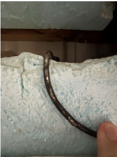
Antenna cable showing locations where the insulation is damaged
