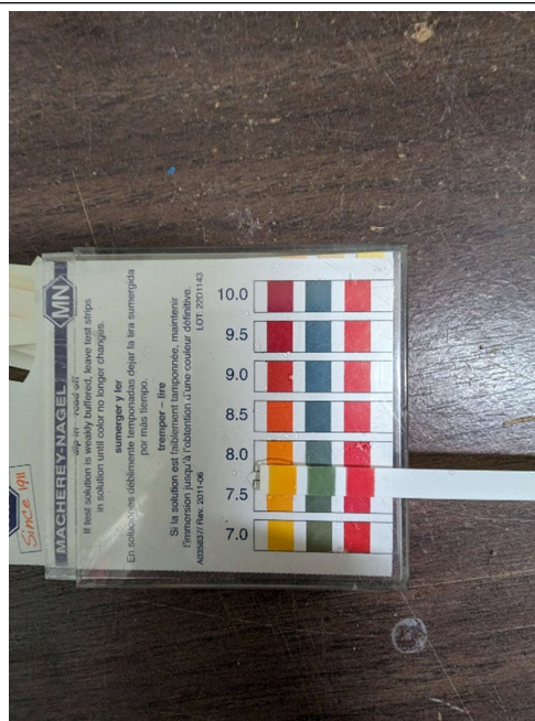
pH strips indicate an effluent pH between 7 and 8.
