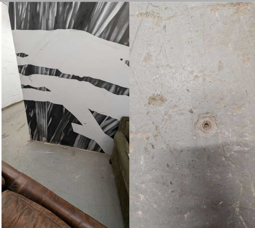
Photo 8: Port-1 in main hallway. Underneath leather couch. Vacuum = 0.000 inWC
