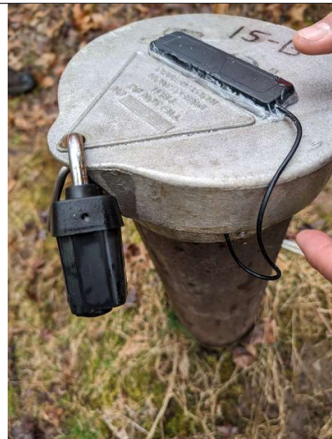
Antenna Installed on MW-15B. Must be Careful when Removing Well Lid.
