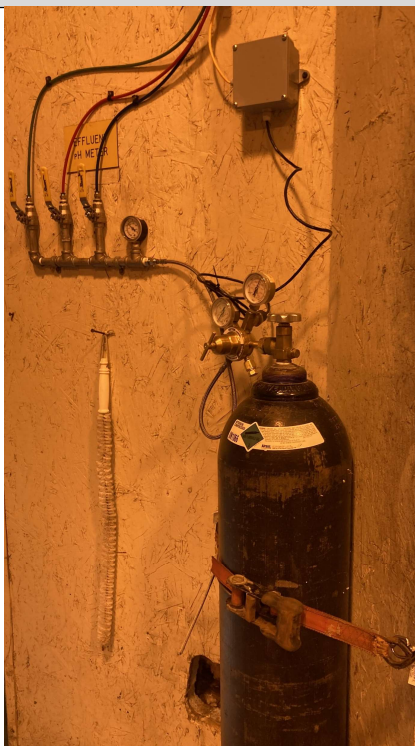
Photo 9: Centralized Nitrogen Source, Pressure Sensor and Manifold for Inflating the Packers.
