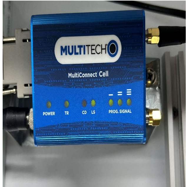
Cell modem located in the control cabinet, power line is the bottom left connection and the antenna connects at the top right.
