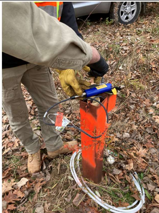
Photo 14: Pilot Test Monitoring Well Data Logger Data Collection
