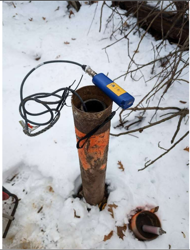
Monitoring Well Level Data Logger Download. (MW-4)
