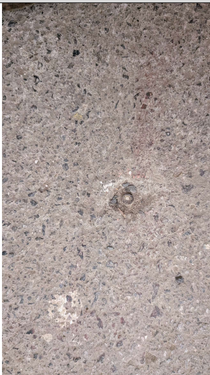
Photo 6: SGP-8. Northern overhead door on west side of the building. Vacuum = 0.000 inWC
