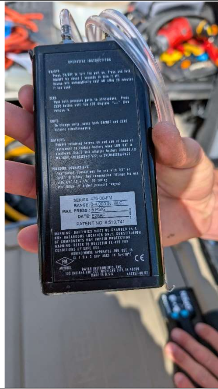
Monometer used for SSDS vacuum readings
