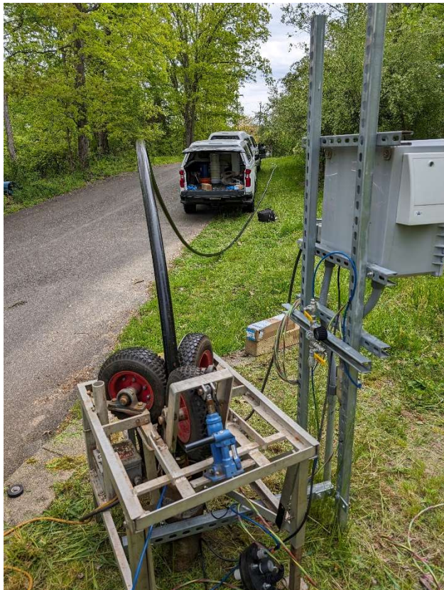
Pump Puller being used to pull pump at MW-5R
