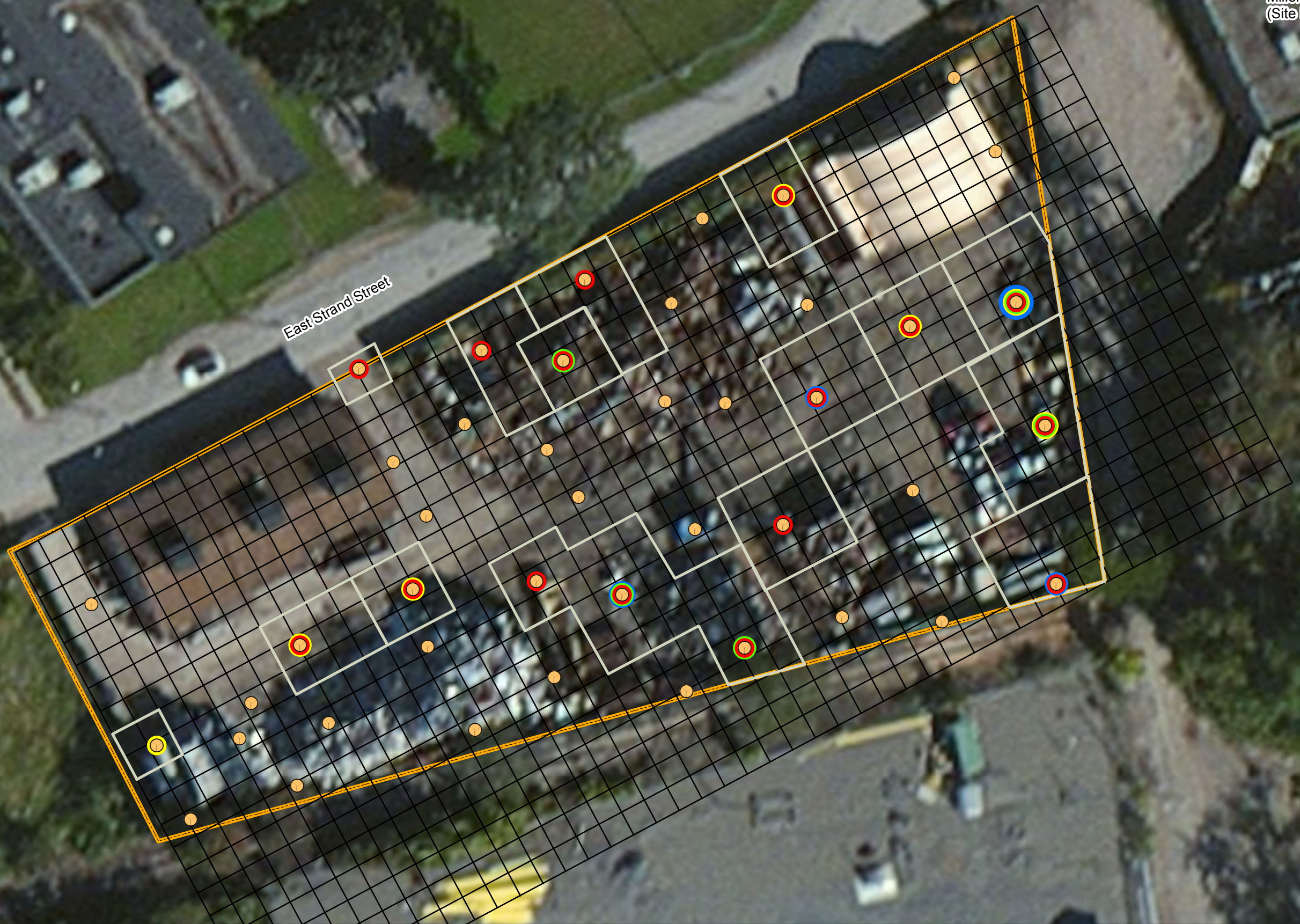
FIGURE 3-1 INTERPRETED HORIZONTAL EXTENT OF CONTAMINATED SOIL/FILL
