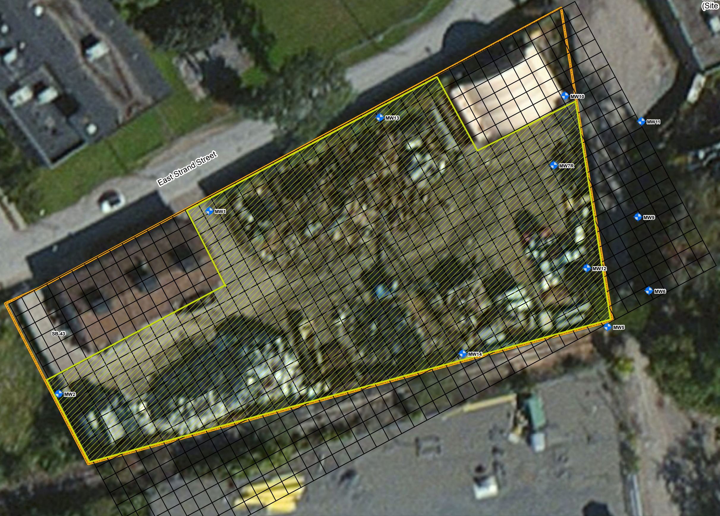
FIGURE 6-1 ALTERNATIVE 3 SOIL COVER, MONITORED NATURAL ATTENUATION OF GROUNDWATER
