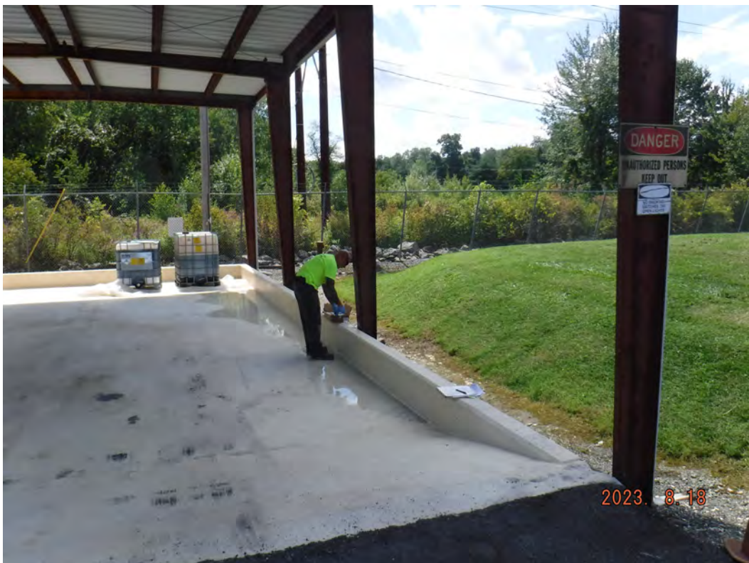
COLLECTING WIPE SAMPLE A3 STRUCTURE (1')
