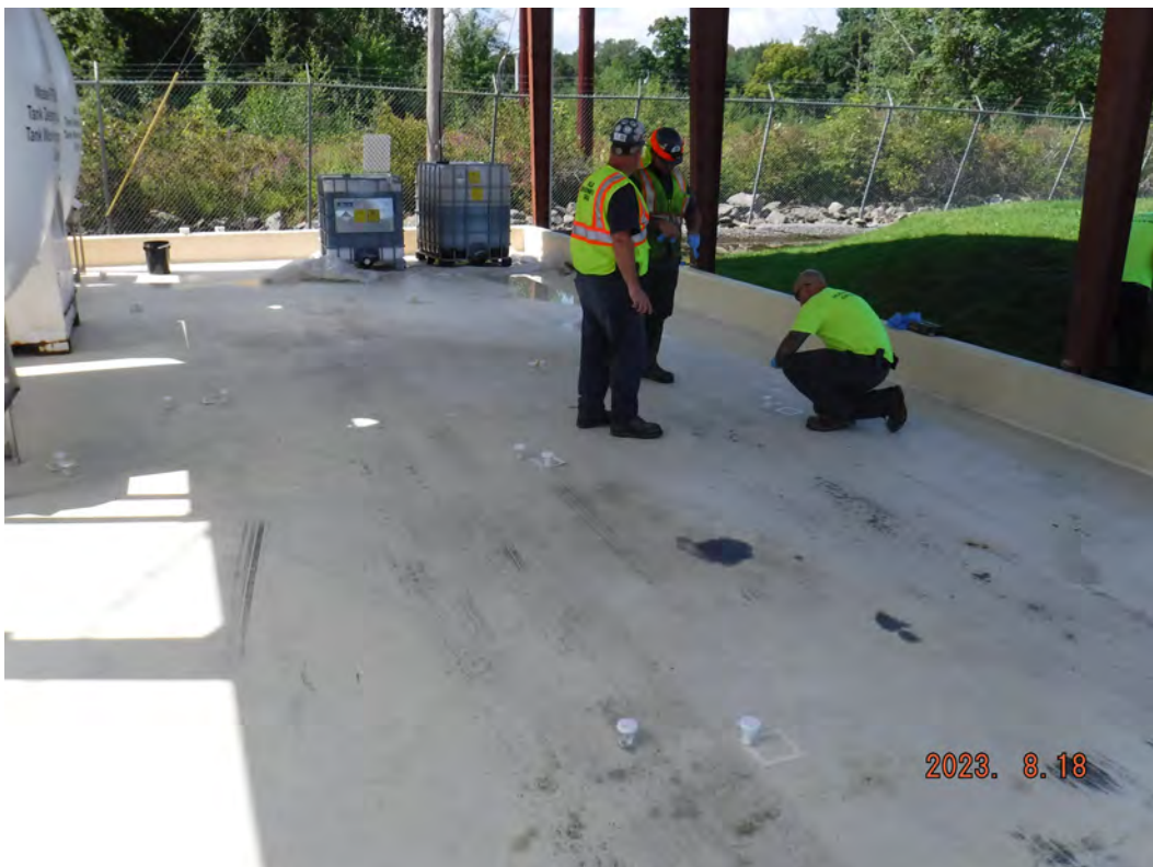
COLLECTING WIPE SAMPLES IN LOADING / UNLOADING AREA
