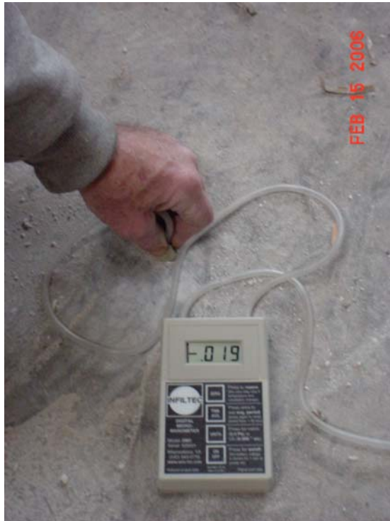
Photo 18 - Measurement of negative pressure under concrete floor using micromanometer.
