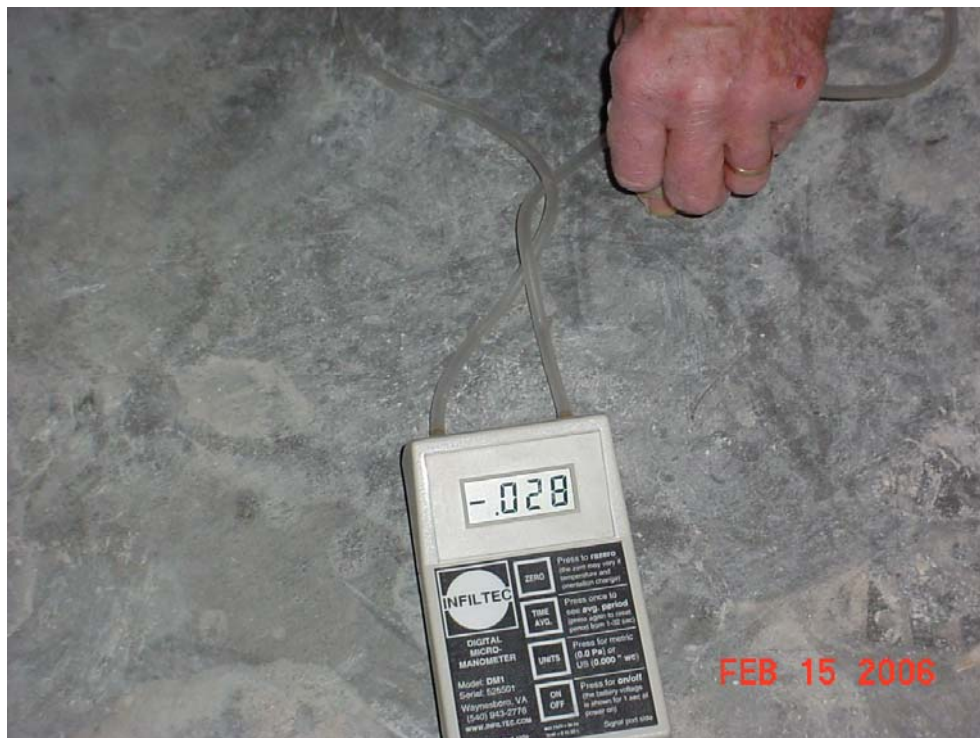
Photo 19 - Measurement of negative pressure under concrete floor using micromanometer.
